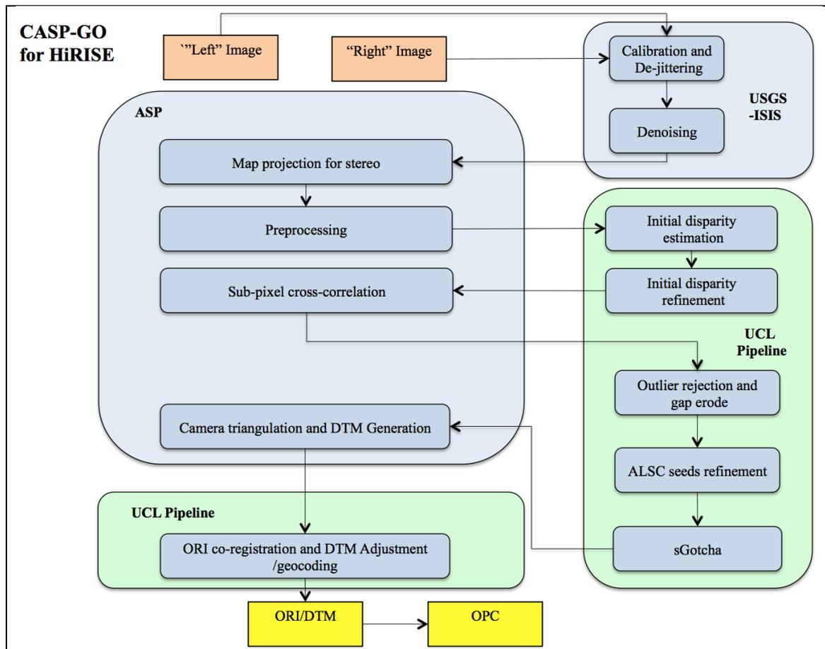
**Figure 1: Flow diagram of the original CASP-GO auto-DTM processing chain and its variation for HiRISE processing.**
