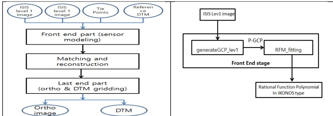
Figure 2: Outlines of UoS stereo processor (left) and sensor modelling part.
