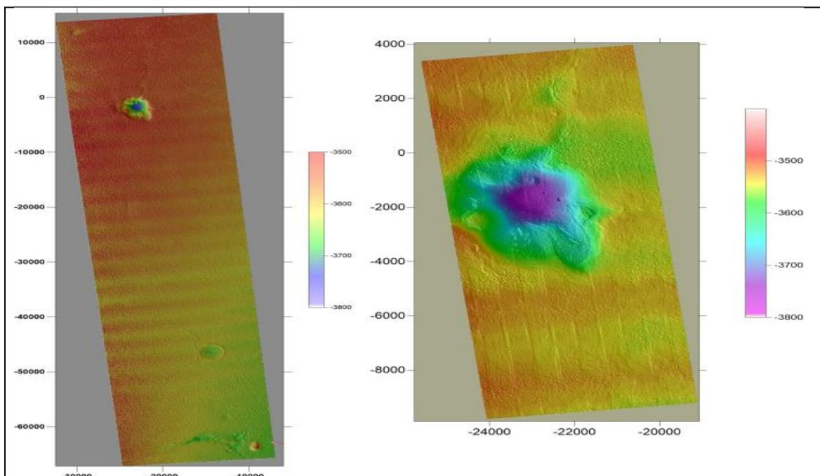
Figure 9: CTX and HiRISE DTMs over the Elysium target area. Note the obvious jitter effect over both CTX (left) as well as HiRISE.
